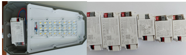
Fig. 1. LED street luminaire and drivers under investigation
