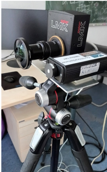
Figure 3a: Measurement setup with the LMK 5 and JETI spectroradiometer
